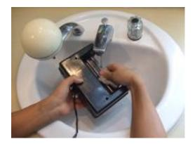
(6) Dry the core by gently wiping it with soft cloth. Or let it stand until it is dried by the air.(7) Place the Singlet core unit back inside its supporting holder.
