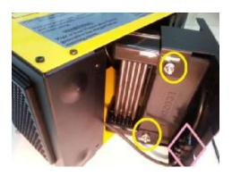
(5) Unscrew the two nuts shown in yellow circles above. This disconnects the Singlet core from its holder. Pull out the screws and gently remove the Singlet core. The result is shown below.
