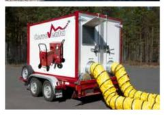
Major costs can be avoided if the drying process is started quickly and in an effective way. Adsorption dehumidifier CTR 10000 is suitable for large new buildings or major water damage. On a trailer it is always ready for rapid deployment.
