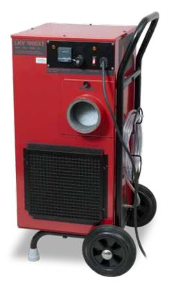
The machine automatically pumps out the condensation water, to a maximum pump height of 4 metres. It also dehumidifies at low temperatures and supplies the room with 3 kW of heat during operation, despite a low energy consumption of only 1.7 kW. CTR LKV 1000XT has a capacity of 20 I/day.
